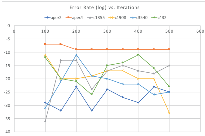
Fig. 9. The error rate of temporary keys generated by Double DIP with increasing of iterations.
